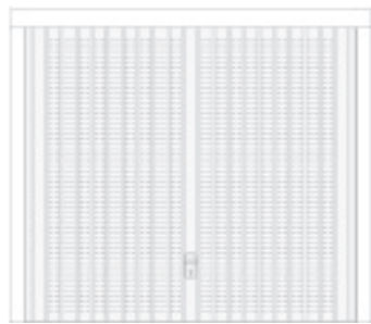
TIPO 9 - TYPE 9 aerazione/sup. porta 12,5% - 15% circa aeration/door surface 12.5% - 15% approx.
