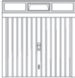
sopraluce fisso con apertura a wasistas centrale fixed fan light with central tilting opening
